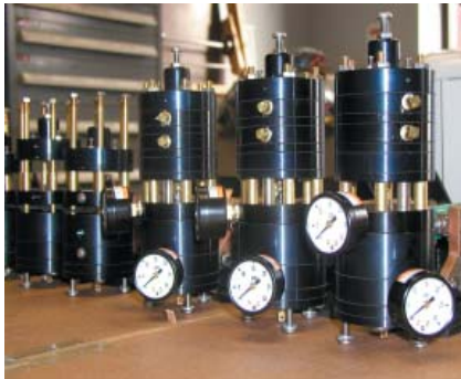
A closer look at the pilot valve control units.
